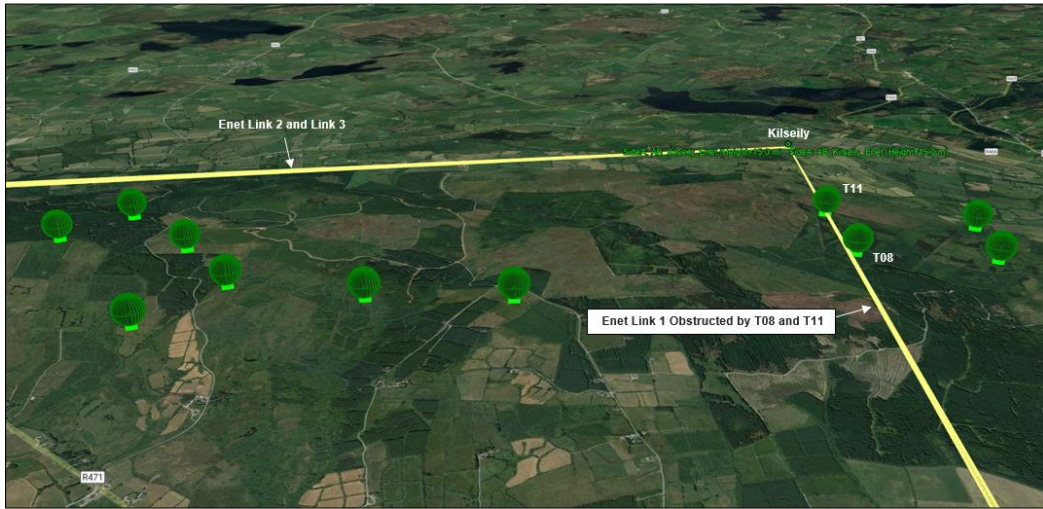
Figure 10. Enet Network – 3D View.
